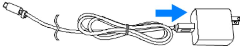
2. Connect the Micro-USB cable to the Micro-USB port on the Tablet PC
